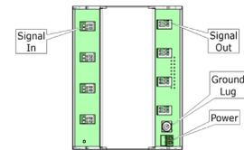
The figure above indicates the input, output and power polarity of the IsoBlock module.
